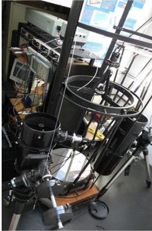
Imagen del prototipo Lidar Multispectral (MSLIDAR) de 40 canales extraída del trabajo “Pawelko Ezequiel et al., 2017: CALBUCO VOLCANIC ASH MEASUREMENTS IN BUENOS AIRES DURING APRIL 2015, 28th ILRC (International Laser Radar Conference), Bucharest, Rumania”; “Pawelko Ezequiel et. al., 2015: MULTISPECTRAL LIDAR TO STUDY THE ATMOSPHERIC AEROSOLS COMPOSITION: MEASUREMENTS IN BUENOS AIRES OF ASHES FROM VOLCANO CALBUCO; International conference on the Atmospheric Sciences and Application to Air Quality (ASAAQ), 13th. KOBE, JAPAN, 2015.”
